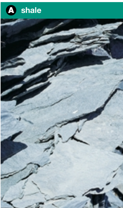
Figure 5.11A Shale, or mudstone, is sedimentary rock formed from fine grains of clay or mud.
