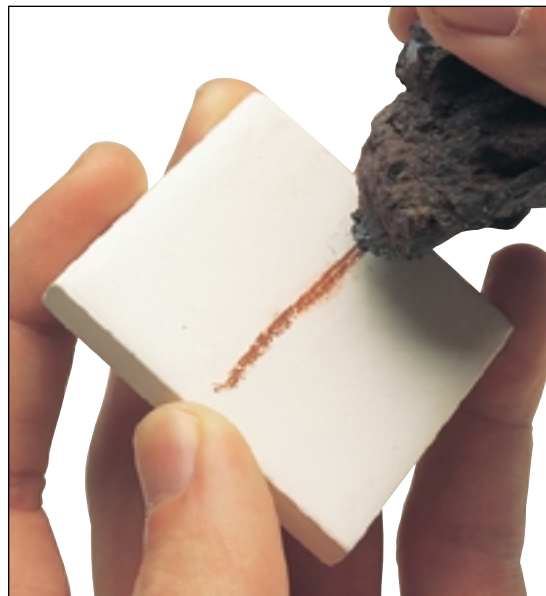
Figure 5.4 Colour is not always useful for mineral identification. Hematite, for example, can be dark red, grey, or silvery in colour. Its streak, however, is always dark red-brown.
