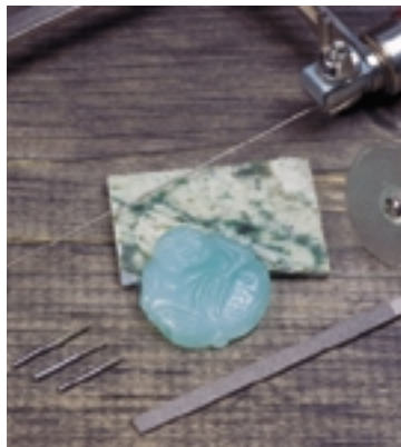
Figure 5.2 Although the glass-cutter wheel looks like ordinary metal, its edge is actually embedded with a hard mineral, such as diamond.
