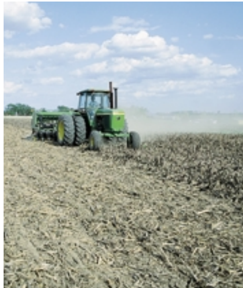
Figure 2.63A In zero tillage, the stubble from last year’s crop remains on the field. A zero-tillage seed drill, like the one shown here, plants the seeds through the stubble.
